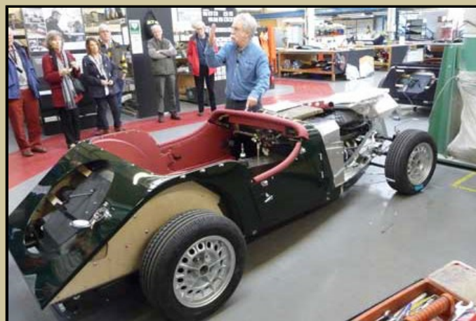
The ash frame is added to the chassis, and wings and trim are put on. Any colour scheme can be chosen.
