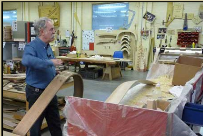
Laminated ash for the curved parts of the wooden frame is shaped by heating in a jig.
