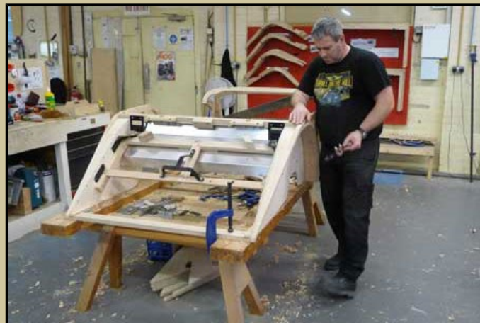
The wooden frame is assembled by hand and finished with a traditional spokeshave and sandpaper.
