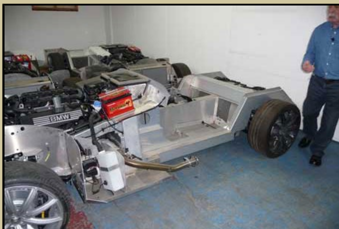
On the larger models the box chassis and panels are aluminium joined by adhesive.
